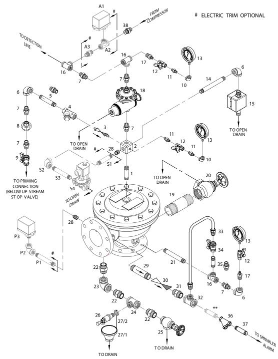
NOTE: WHEN ELECTRIC TRIM IS SUPPLIED THEN SL.NO.28 PLUG NOT REQUIRED.
