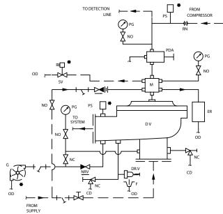
Electric & Hydraulic Release Trim - Schematic Deluge Valve Model - A Size 50 / 80 / 100 / 150 / 200 DN
