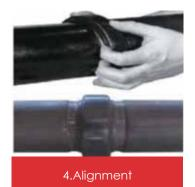
After aligning two pipe ends together, pull the gasket into position, centering between the grooves on each pipe. The gasket should not extend into the groove on either pipe.
