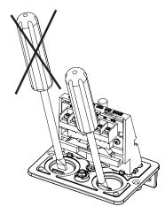
NOTE: Do not drill into the base as this creates metal shavings which can create electrical hazards and damage the device. Drilling voids the warranty.
